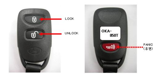
You can lock and unlock your vehicle with the remote transmitter.
