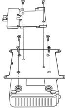
Mounting screws for this wireless unit must be tightened with torque of 4.4 to 5.3 in. lb. (0.5 to 0.6 N.m)
