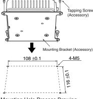
Mounting Hole Process Drawing (Unit: mm)
