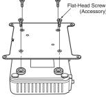
Mounting screws for this wireless unit must be tightened with torque of 4.4 to 5.3 in. lb. (0.5 to 0.6 N.m)
