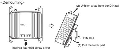
under the lower tab and pull downward
