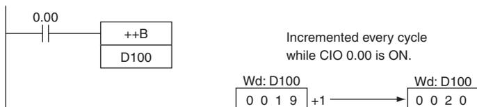
In the following example, the 8-digit BCD content of D101 and D100 will be incremented by 1 every cycle as long as CIO 0.00 is ON.
