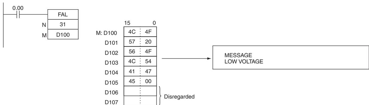
**Note** If two or more errors occur at the same time, the error code of the most serious error (with the highest error code) will be stored in A400.
