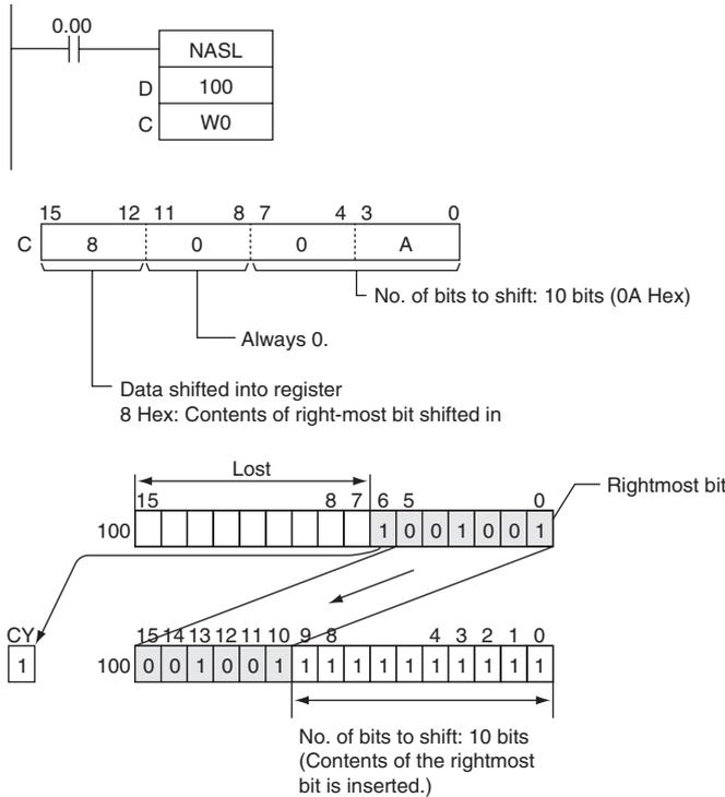
When CIO 0.00 is ON, CIO 100 and CIO 101 will be shifted to the left (from the rightmost bit to the leftmost bit) by 10 bits. The number of bits to shift is specified in bits 0 to 7 of W0 (control data). The contents of bit 0 of CIO 100 is copied into bits from which data was shifted and the contents of the rightmost bit which was shifted out of range is shifted into the Carry Flag (CY). All other data is lost.
