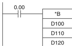
When CIO 0.00 is ON in the following example, D100 and D110 will be multiplied as 4-digit BCD values and the result will be output to D121 and D120.
