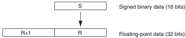
Only values within the range of -32,768 to 32,767 can be specified for S. To convert signed binary data outside of that range, use FLTL(453).
