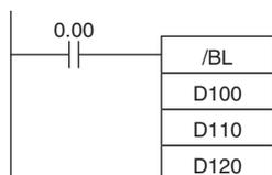
When CIO 0.00 is ON in the following example, D101 and D100 will be divided by D111 and D110 as 8-digit BCD values and the quotient will be output to D121 and D120 and the remainder to D123 and D122.
