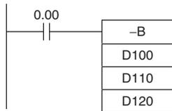
When CIO 0.00 is ON in the following example, D110 is subtracted from D100 as 4-digit BCD values, and the result will be output to D120.
