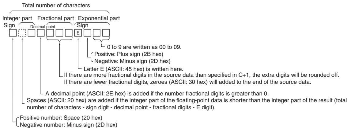
**Note** Either one or two bytes of zeroes are added to the end of ASCII text as an end code.
