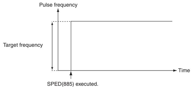
In independent mode, pulse output will stop automatically when the number of pulses set with PULS(886) in advance have been output. In continuous mode, pulse output will continue until stopped from the program.
