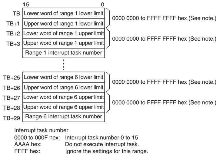
**Note** Always set the upper limit greater than or equal to the lower limit for any one range.
