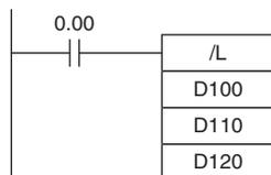
When CIO 0.00 is ON in the following example, D101 and D100 are divided by D111 and D110 as 8-digit signed hexadecimal values and the quotient will be output to D121 and D120 and the remainder to D123 and D122.
