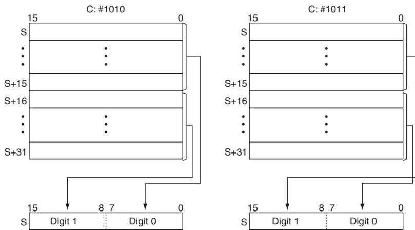
If the conversion data contains 0000 hex, but other data is to be encoded, separate the conversion by using more than one DMPX(077) instructions.
