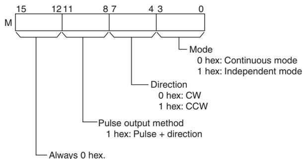
**Note** Use the same pulse output method when using both pulse outputs 0 and 1.
