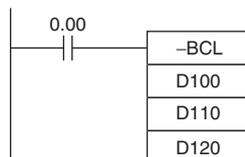
When CIO 0.00 is ON in the following example, D111, D110, and CY will be subtracted from D101 and D100 as 8-digit BCD values, and the result will be output to D121 and D120.
