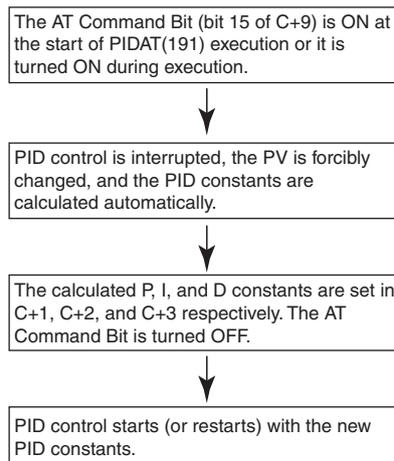
**Note 1** If autotuning is interrupted by turning OFF the AT Command Bit during autotuning, PID control will start with the PID constants that were being used before autotuning began.
