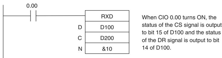
When CIO 0.00 turns ON, the status of the CS signal is output to bit 15 of D100 and the status of the DR signal is output to bit 14 of D100.
