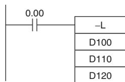
When CIO 0.00 is ON in the following example, D111 and D110 will be subtracted from D101 and D100 as 8-digit signed binary values and the result will be output to D121 and D120.
