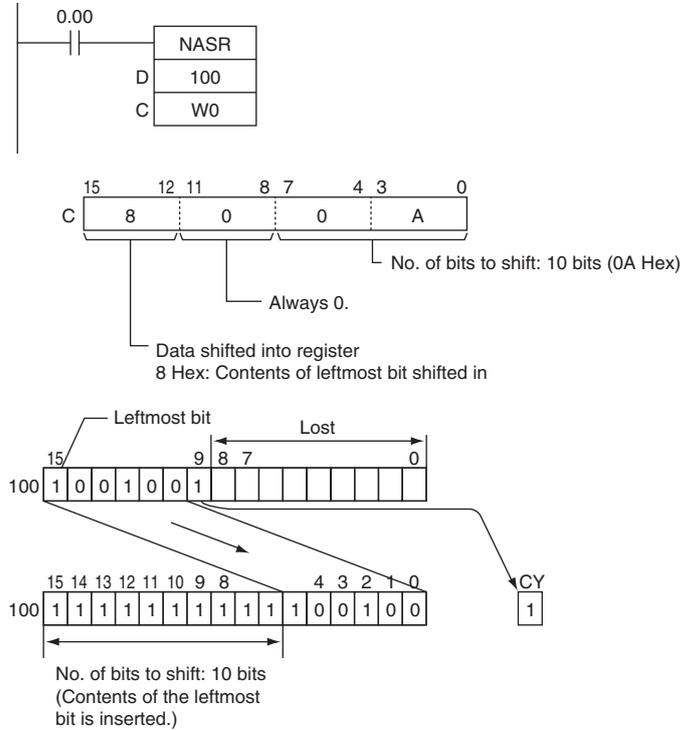
When CIO 0.00 is ON, CIO 100 and CIO 101 will be shifted 10 bits to the right (from the leftmost bit to the rightmost bit). The number of bits to shift is specified in bits 0 to 7 of W0 (control data). The contents of bit 15 of CIO will be copied into the bits from which data was shifted and the contents of the leftmost bit of data which was shifted out of range will be shifted into the Carry Flag (CY). All other data is lost.
