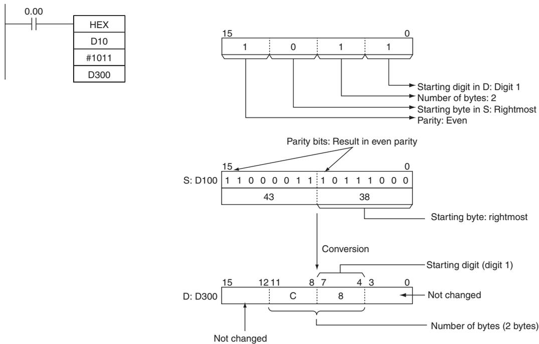
● Example of converting multiple bytes of ASCII code to hex
