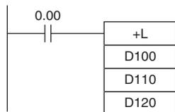
When CIO 0.00 is ON, D101 and D100 and D111 and D110 will be added as 8-digit signed binary values and the result will be output to D121 and D120.
