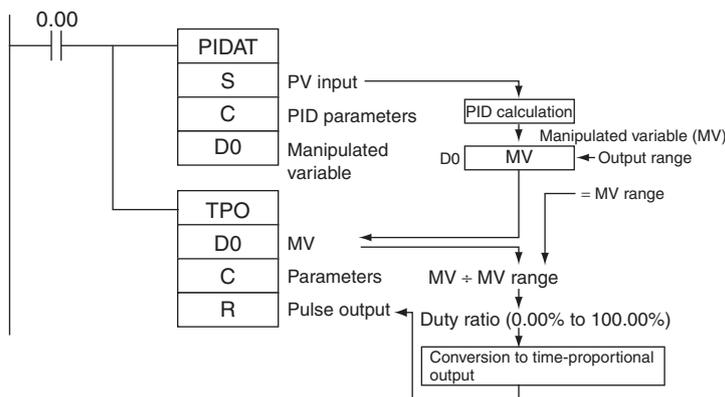
In this case, set the same value for the PID Control instruction's output range and the TPO(685) instruction's manipulated variable range. For example, when the PID Control instruction's output range and the TPO(685) instruction's manipulated variable range are both set to 12 bits (0000 to 0FFF hex), the duty ratio is calculated by dividing the manipulated variable from the PID Control instruction by 0FFF hex and TPO(685) converts that duty ratio to a time-proportional output.
