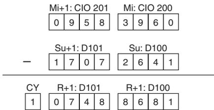
The Carry Flag (CY) will be turned ON, so the actual number is - 7,488,681. Because the content of D101 and D100 is negative, CY is used to turn ON CIO 21.00 to indicate this.
