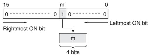
As shown at right, 256 to 8 encoding consists of converting the bit number (m) of the leftmost or rightmost bit that has 1 set among the 256 bits to an 8-bit binary value.
