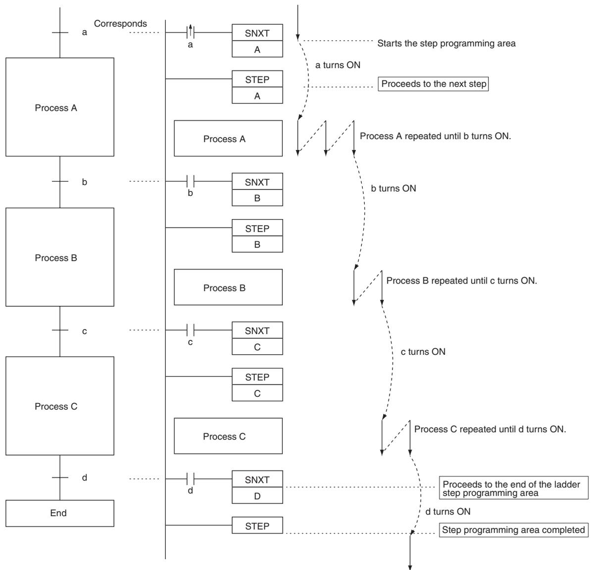
**Note** Work bits are used as the control bits for A, B, C and D.
