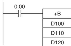
When CIO 0.00 is ON in the following example, D100 and D110 will be added as 4-digit BCD values, and the result will be output to D120.
