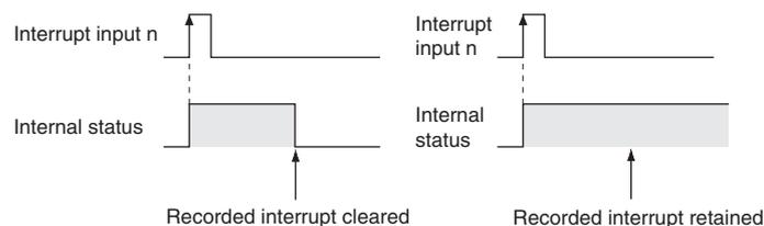
If an I/O interrupt task is being executed and an interrupt input with a different interrupt number is received, that interrupt number is recorded internally. The recorded I/O interrupts are executed later in order of their priority (from the lowest number to the highest).
