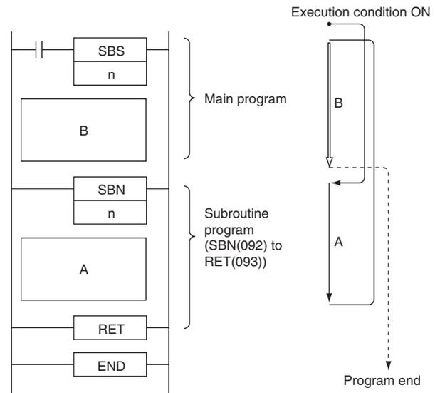
Subroutines can be nested up to 16 levels. Nesting is when another subroutine is called from within a subroutine program, such as shown in the following example, which is nested to 3 levels.
