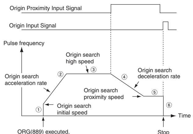
When the origin search operation has been completed, the Error Counter Reset Output will be turned ON.
