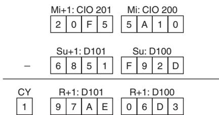
The Carry Flag (CY) is turned ON, so the actual number is -97AE06D3. Because the content of D101 and D100 is negative, CY is used to turn ON CIO 21.00 to indicate this.
