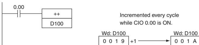
In the following example, the content of D100 will be incremented by 1 every cycle as long as CIO 0.00 is ON.
