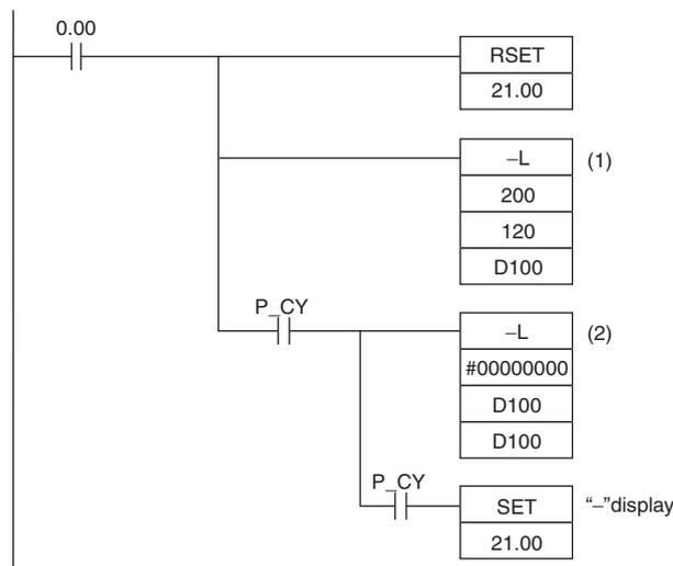
In this example, the eight-digit binary value in CIO 121 and CIO 120 is subtracted from the value in CIO 201 and CIO 200, and the result is output in eight-digit binary to D101 and D100. If the result is negative, the instruction at (2) will be executed, and the actual result will then be output to D101 and D100.
