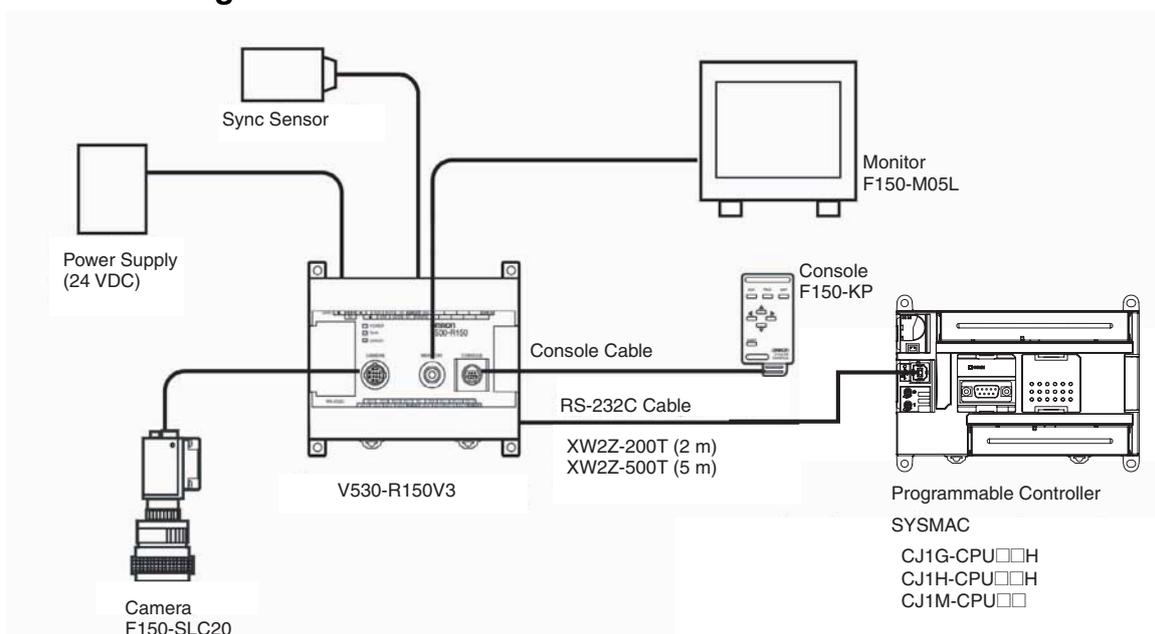
In this example, the external device is connected to the RS-232C port built into the CPU Unit.
