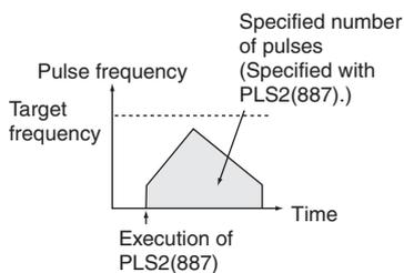
● Switching from Continuous Mode Speed Control to Independent Mode Positioning
