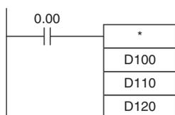
When CIO 0.00 is ON in the following example, D100 and D110 will be multiplied as 4-digit signed hexadecimal values and the result will be output to D120 and D121.
