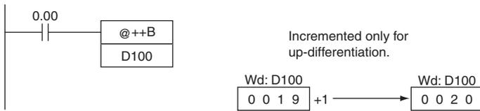
The up-differentiated variation is used in the following example, so the BCD content of D101 and D100 will be incremented by 1 only when CIO 0.00 has gone from OFF to ON.
