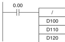
When CIO 0.00 is ON in the following example, D100 will be divided by D110 as 4-digit signed binary values and the quotient will be output to D120 and the remainder to D121.
