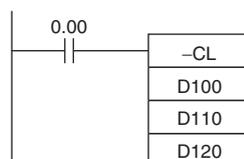
When CIO 0.00 is ON in the following example, D111, D110 and CY will be subtracted from D101 and D100 as 8-digit signed binary values, and the result will be output to D121 and D120.
