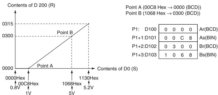
In this example, values from 0000 to 00C8 hexadecimal will be converted to negative values. SCL(194), however, can output only unsigned BCD values from 0000 to 9999, so 0000 BCD will be output whenever the contents of D0.00 is between 0000 and 00C8 hexadecimal.
