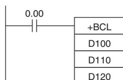
When CIO 0.00 is ON in the following example, D101, D100, D111, D110, and CY will be added as 8-digit BCD values, and the result will be output to D121 and D120.
