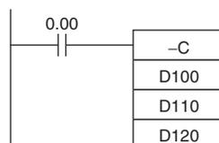
When CIO 0.00 is ON in the following example, D110 and CY will be subtracted from D100 as 4-digit signed binary values and the result will be output to D120.
