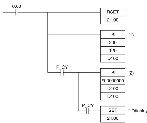
In this example, the eight-digit BCD content of CIO 121 and CIO 120 is subtracted from the content of CIO 201 and CIO 200, and the result is output in eight-digit BCD to D101 and D100. The result is negative, so the instruction at (2) will be executed, and the true value will then be output to D101 and D100.
