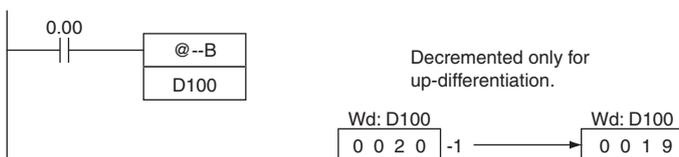
The up-differentiated variation is used in the following example, so the BCD content of D101 and D100 will be decremented by 1 only when CIO 0.00 has gone from OFF to ON.
