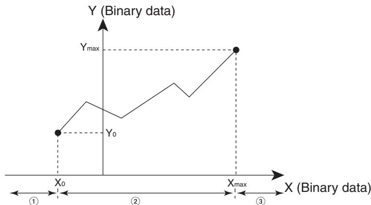
Up to 256 endpoints can be stored in the line-segment data table beginning at C+1.
