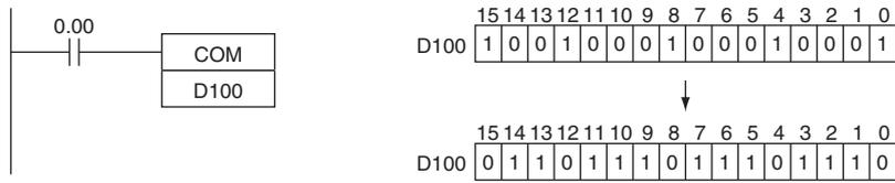
When CIO 0.00 is ON in the following example, the status of each bit in D100 and D101 will be reversed.
