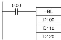
When CIO 0.00 is ON in the following example, D111 and D110 will be subtracted from D101 and D100 as 8-digit BCD values, and the result will be output to D121 and D120.
