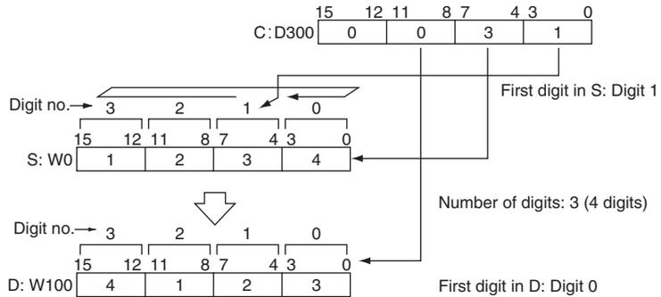
**Note** After reading the leftmost digit of S (digit 3), MOVD(083) wraps to the rightmost digit (digit 0).
