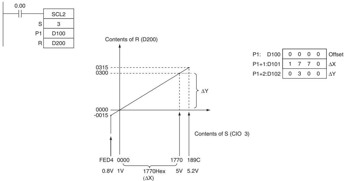
● **Scaling 1 to 5-V Analog Input to -200 to 200**
