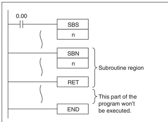
**Note** The input method for the subroutine number, N, is different for the CX-Programmer. Input #0 to #127 on the CX-Programmer.
