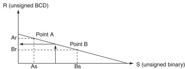
Reverse scaling can be used, for example, to convert (reverse scale) 1 to 5 V (0000 to 0FA0 hexadecimal) to 0300 to 0000, respectively, as shown in the following diagram.
