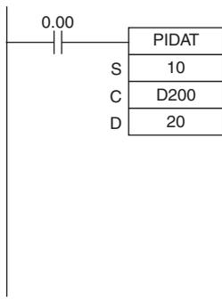
At the rising edge of CIO 0.00 (OFF to ON), autotuning will be performed first if bit 15 of D209 (C+9) is ON. When autotuning is completed, the calculated P, I, and D constants are written to C+1, C+2, and C+3. PID control is then started with the calculated PID constants.
