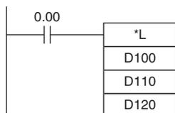
When CIO 0.00 is ON in the following example, D101, D100, D111, and D110 will be multiplied as 8-digit signed hexadecimal values and the result will be output to D123, D122, D121 and D120.
