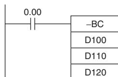
When CIO 0.00 is ON in the following example, D110 and CY will be subtracted from D100 as 4-digit BCD values, and the result will be output to D120.
