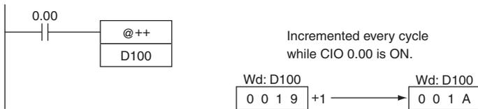
The up-differentiated variation is used in the following example, so the content of D101 and D100 will be incremented by 1 only when CIO 0.00 has gone from OFF to ON.
