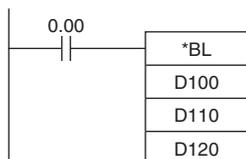
When CIO 0.00 is ON in the following example, D101, D100, D111, and D110 will be multiplied as 8-digit unsigned BCD values and the result will be output to D123, D122, D121 and D120.
