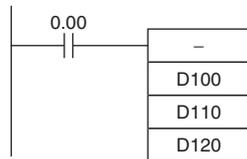
When CIO 0.00 is ON in the following example, D110 will be subtracted from D100 as 4-digit signed binary values and the result will be output to D120.
