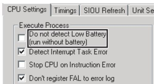
**Note** Even if PLC Setup word 129 bit 15 is set to 1 (Do not record FAL Errors in Error Log.), the following errors will be recorded:
