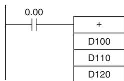
When CIO 0.00 is ON in this example, D100 and D110 will be added as 4-digit signed binary values and the result will be output to D120.
