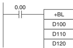
When CIO 0.00 is ON in the following example, D101 and D100 and D111 and D110 will be added as 8-digit BCD values, and the result will be output to D121 and D120.
