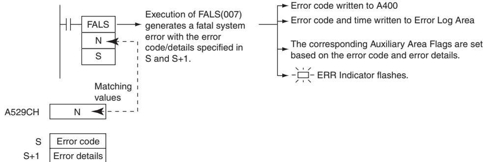
When FALS(007) is executed with N set to an FAL number (1 to 511) that is equal to the content of A529 (the system-generated FAL/FALS number), a fatal error will be generated with the error code and error details code specified in S and S+1. The following processing will be performed at the same time:
