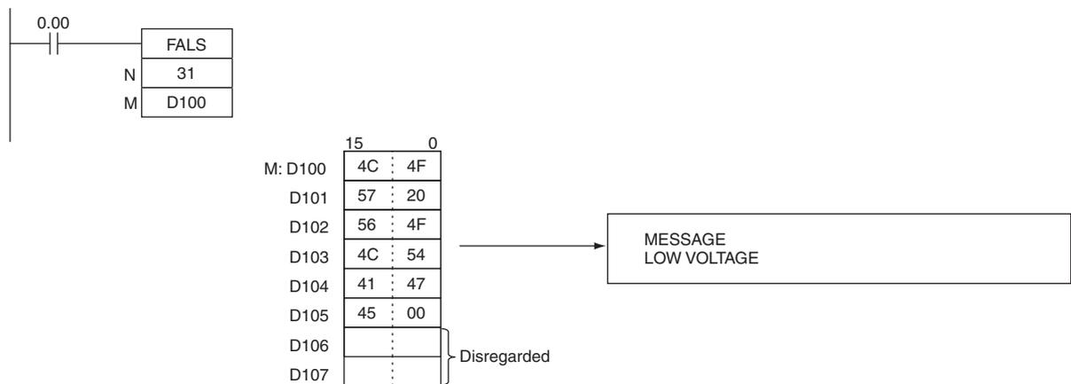
**Note** A400 will contain the error code of the most serious of all of the errors that have occurred, including non-fatal and fatal system errors, as well as errors generated by FAL(006) and FAL(007).
