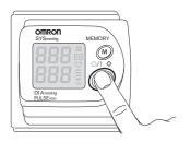
2 Press Memory Recall button for latest and previous values. Press On/Off button to turn off power. Note: Display shows alternately blood pressures and heartbeats.
