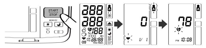
**NOTE:** To stop the inflation or measurement, press the START/STOP button. The monitor will stop inflating, start deflating and will turn off.
