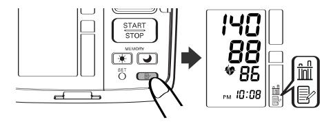
3. Press the Memory button ( ) to display the most recent set of measurement values on the screen. The values are displayed from the most recent to the oldest.
