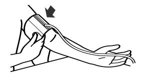
6. Apply the cuff to your left upper arm so the blue strip is on the inside of your arm and aligned with your middle finger. The air tube runs down the inside of your arm. The bottom of the cuff should be approximately 1/2" above your elbow.
