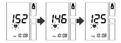
4. When the measurement is complete, the arm cuff completely deflates. Your blood pressure and pulse rate are displayed.
