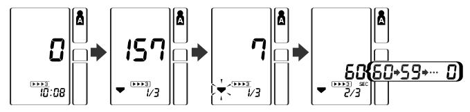
The second measurement is complete, waiting to start the next measurement.
