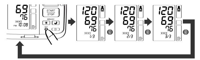
4. Press the START/STOP button to turn the power off.
