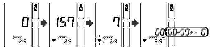
The consecutive measurements are complete. The average for three measurements appears on the display.
