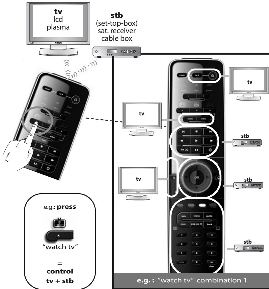
**Example 1 (configuration as shown):****How to activate "watch tv" combination 1**
