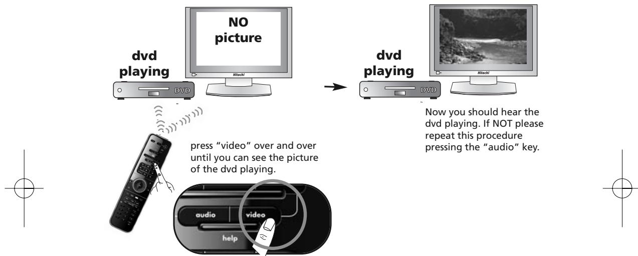
**If the "help" function is NOT working it needs to be activated.****E.g. How to activate the "help" function for finding the video (or audio for amp/mp3) -input in SmartControl in "watch tv" mode.**
