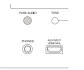
Selecting Pure Audio for listening mode turns off the display and analog video circuitry, but the video signals input through HDMI input are output from HDMI output.
