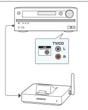
Connect an Onkyo component with RI jack to this unit using an RI cable and an analog audio (RCA) cable. For details, refer to the instruction manual of the component with RI jack. The RI cable can be connected in any order. When there are two RI jacks, both jacks work in the same way and are interchangeable.
