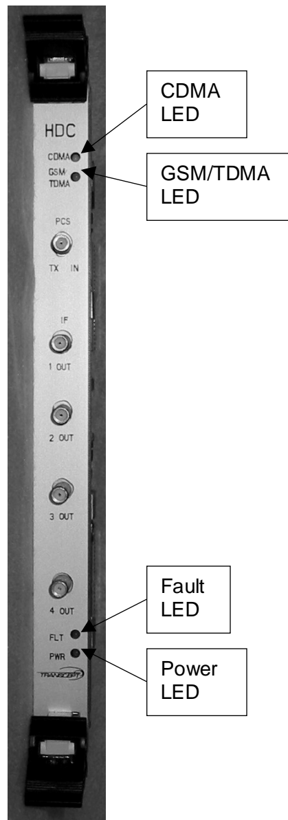
Figure 15. Hub Down Converter Front Panel
