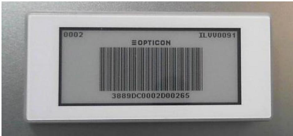
The EE-292 is an e-paper based electronic shelf label with a screen size of 2.9". It has a build-in NFC reader plus several 3-color LEDs.
