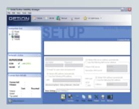
In **PDP type** you can specify the PDP type. You can choose between IP and PPP. If required by your carrier you have to fill in the address. (Typically the connection is type IP).
