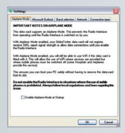
a) If you tick <Enable Airplane Mode at Startup>, the card's radio will be powered down. Therefore, as specified into the pop up, the card will not register and you will not be able to make an Internet dial up connection or send/receive SMS.
