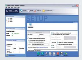
In **PDP type** you can specify the PDP type. You can choose between IP and PPP. If required by your carrier you have to fill in the address. (Typically the connection is type **IP**).
