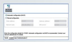
The check box in the page determines whether the other controls are activated. If "Automatic configuration (DHCP)" is on, the other settings cannot be modified. In this case the AP configures TCP/IP automatically.
