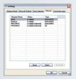
To check the current settings and read the current list of networks, click **Query**. The list displays all available networks. The operator's status is shown in the second column. To register with a different operator, highlight the Operator name, click **Select** and click **OK** Selecting an operator switches the GlobeTrotter to manual registration mode; it will try to register with the selected operator only. To go back to automatic registration, you must click Automatic.
