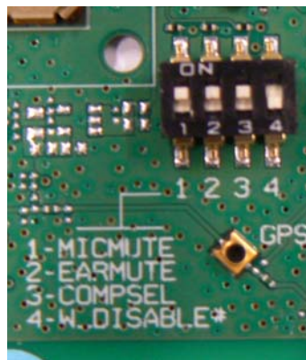
Figure 10: Switch 4 (W. Disable) is in OFF position.
