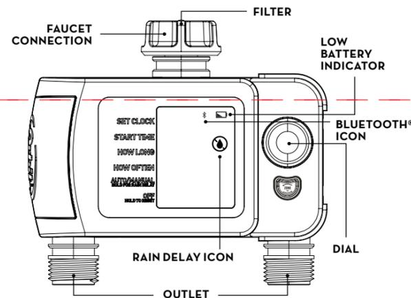
Write down the MAC address: 12 digit alphanumeric code located on the bottom of the timer.
