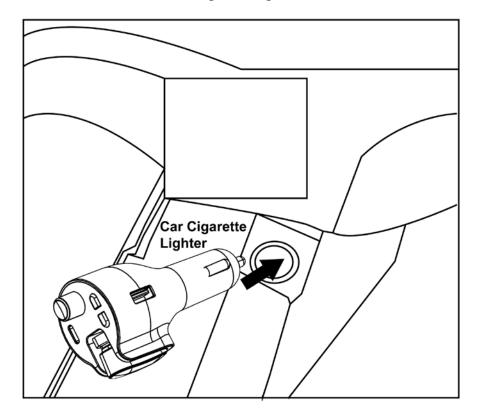
2. The unit will automatically power on and the LED Display on the Unit will illuminate & blink. The voltage of the car battery will appear on the LED Display at first.
