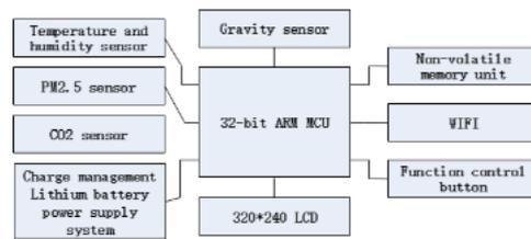
① Sensor module – Sampling the environment data, including laser PM2.5 sensor, Temperature/humidity sensor SHT30, CO2 sensor Senseair-S8, gravity sensor ADXL345.
