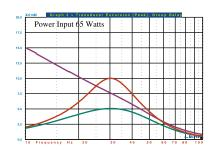
with the filter and with the filter and the INTELLi Q set to +3dB. As you can see with +3dB of boost and the high-pass filter set to 30Hz, the woofer has more output down to 25Hz and less overall excursion when compared to the non-high-pass response. Maximum physical excursion capability of the woofer is 15mm.
