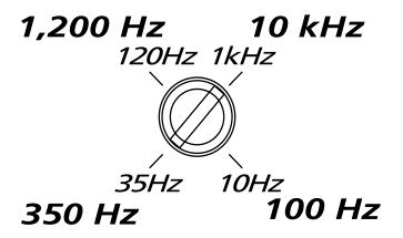
The crossover section is marked at four frequency points for ease of system adjustment. These points are 10 Hz, 35 Hz, 120 Hz and 1 kHz. Specific crossover points can be to be chosen based on the recommended operational bandwidth of your speakers.
