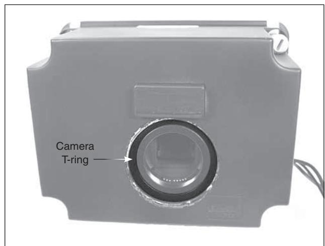
**Figure 4.** With the camera installed, the T-ring on the camera should be seated snugly in the aperture port of the housing.
