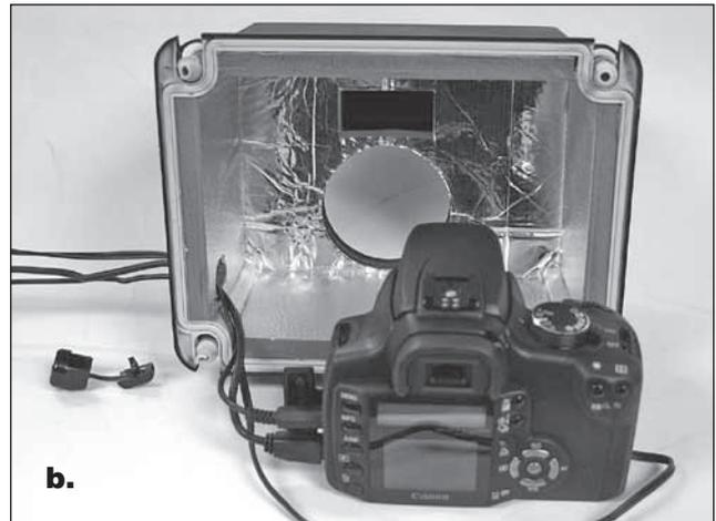
**Figure 3. a)** With the plastic cable collar removed, run your camera cables through the hole in the side of the housing, **b)** plug DC coupler and other cables into the camera before installing the camera in the cooling chamber
