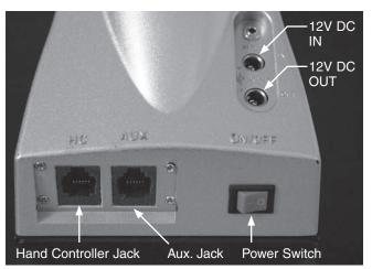
Figure 4b: Connector Ports on the TeleTrack AZ-G GoTo Mount
