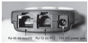
Figure 4a: Hand controller outlets
