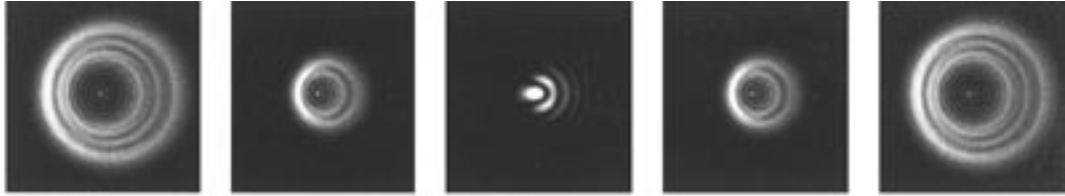
Figure 7. Even though the star pattern appears the same on both sides of focus, it is asymmetric. The dark obstruction is skewed off to the left side of the diffraction pattern indicating poor collimation.
