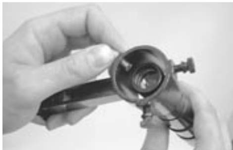
Figure 3c. Pull the spring-loaded tensioner outward, then insert the finder scope into the finder scope bracket.
