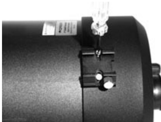
Figure 3a. Attaching the optional dovetail finder scope base.
