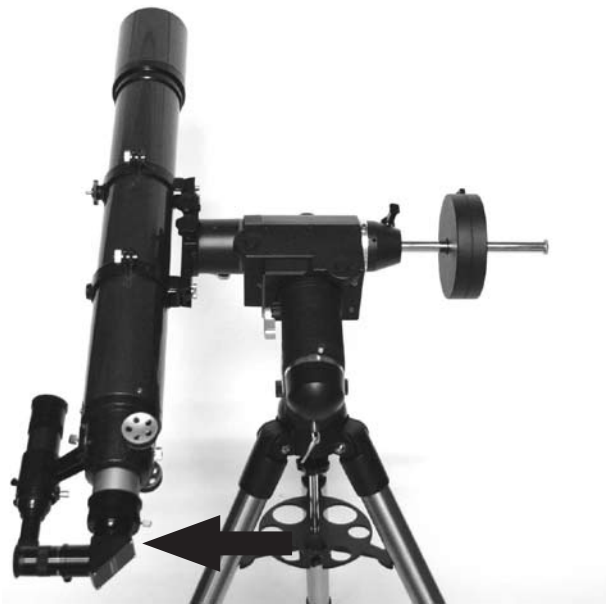
Figure 18. Gently push the telescope horizontally to determine direction of optical axis offset.
