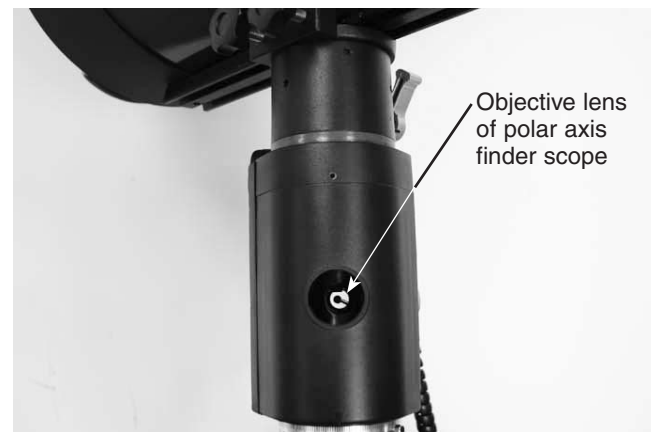
Figure 8. The optical tube must be rotated about the Dec. axis until you have a clear view along the R.A. axis with the polar axis finder scope.
