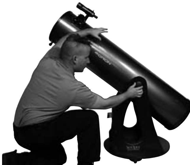
Figure 29. Adjust the tensioning knob until the altitude balance is just right. The telescope should move easily in altitude without drifting when you let go.
