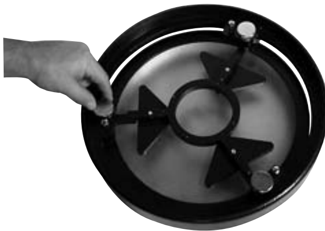
Figure 26. The tilt of the primary mirror is adjusted by turning one or more of the three collimation knobs.
