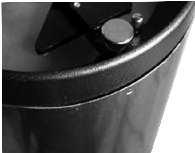
Figure 7. Locate the area of tube that is bulging out and preventing the mirror cell from fully seating.
