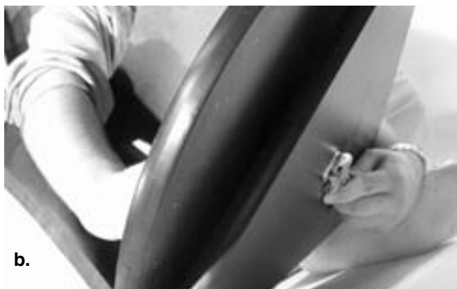
Figure 11. To connect the baseplates, tilt them only slightly, as shown. Do not place them on their side. (a) Use one wrench (or pliers) to hold the hex nut steady (b) while turning the hex head of the azimuth axis screw with another wrench.
