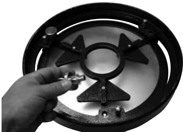
Figure 5. Thread the collimation thumbnuts, with nylon washers attached, through the rear end ring and onto the threaded shafts. Make sure the thumbnuts have at least three full turns of engagement on the shafts.
