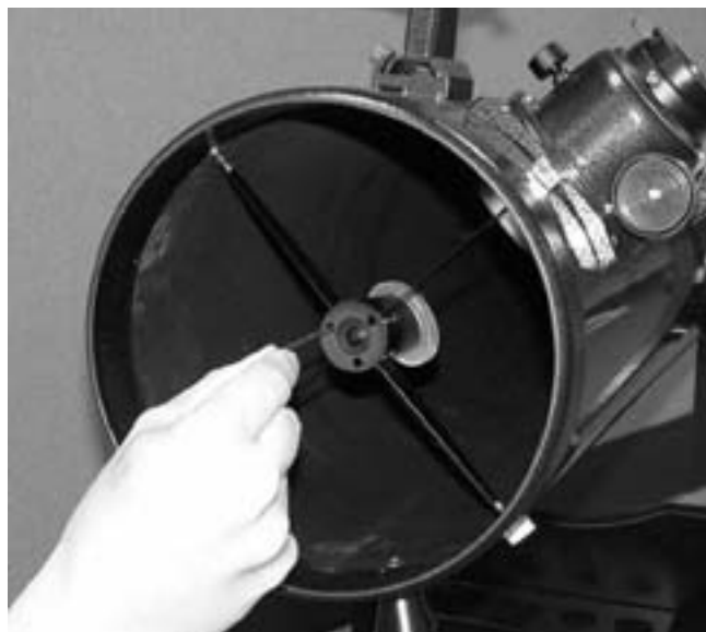
Figure 24. Adjust the tilt of the secondary mirror by loosening or tightening the three alignment set screws with a 2mm hex key.
