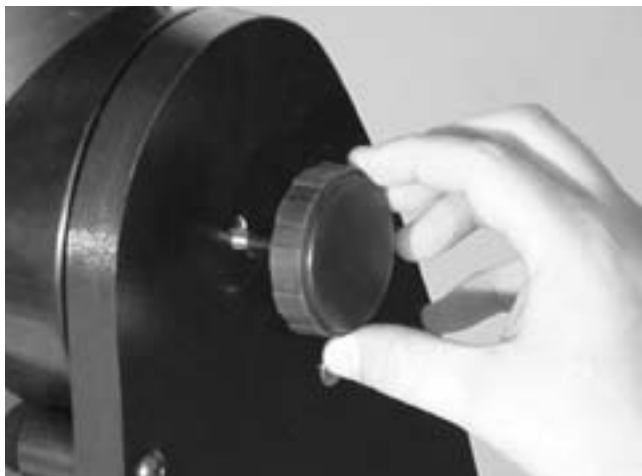
Figure 18. The retaining knob with the nylon spacer is installed on the side of the base that does not have the IntelliScope port.
