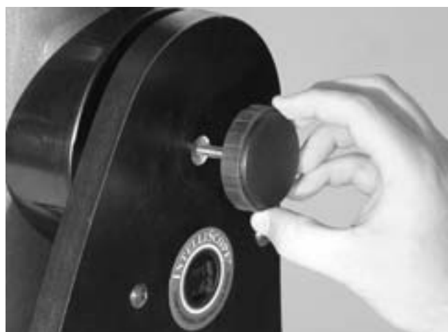
Figure 17. The tensioning knob, with the metal and nylon washers, goes on the side of the base with the IntelliScope port. The tensioning knob should be tightened until the CorrecTension pads just touch the telescope’s altitude bearing.
