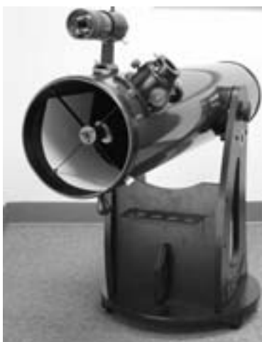
Figure 22. The SkyQuest IntelliScope properly set up for collimation. Note the white paper placed across from the focuser, and the level angle of the optical tube. Ideally, the telescope should be pointing at a white wall.
