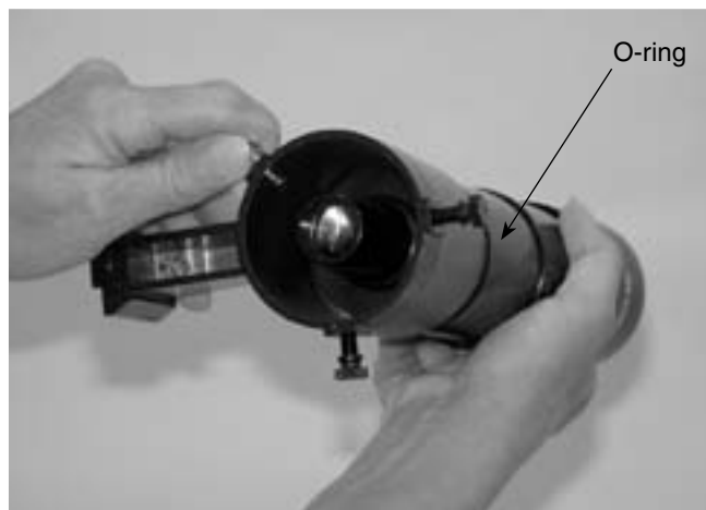
Figure 19b. Pull back on the tensioner and slide the finder scope into its bracket until the O-ring is seated in the bracket's ring.
