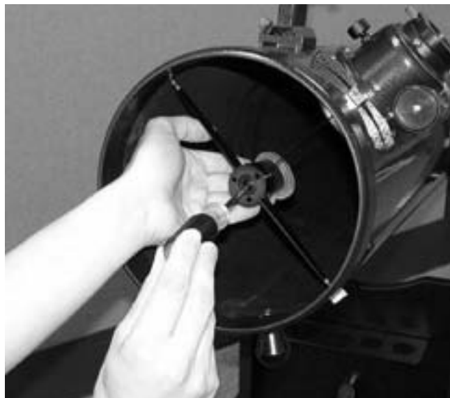
Figure 23. To center the secondary mirror under the focuser, hold the mirror holder in place with one hand while adjusting the center bolt with a Phillips screwdriver. Do not touch the mirror's surface!
