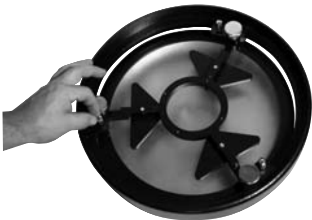
Figure 25. The three small thumbscrews that lock the primary mirror in place must first be loosened before any adjustments can be made.
