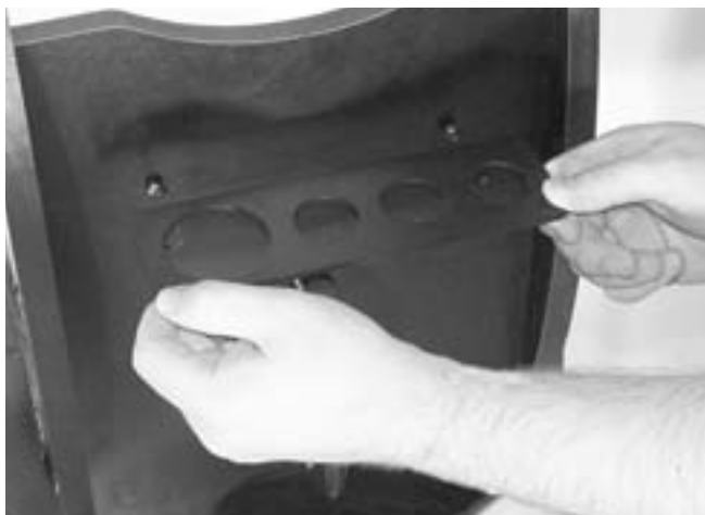
Figure 15. Using the two supplied screws, install the aluminum eyepiece rack in the predrilled holes near the top of the front baseplate.
