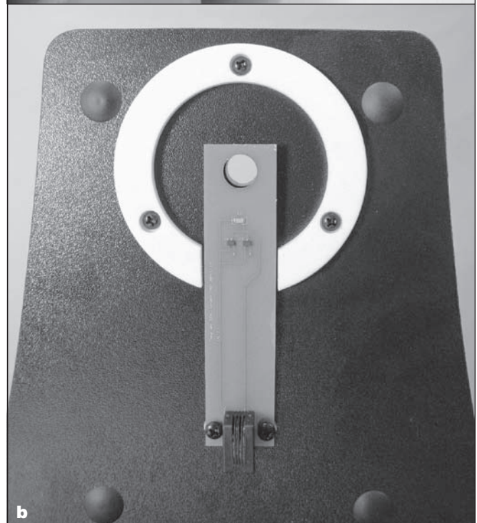
Figure 12. (a) Installing the altitude encoder board. Place a washer on each screw, as shown. (b) The altitude encoder board installed.
