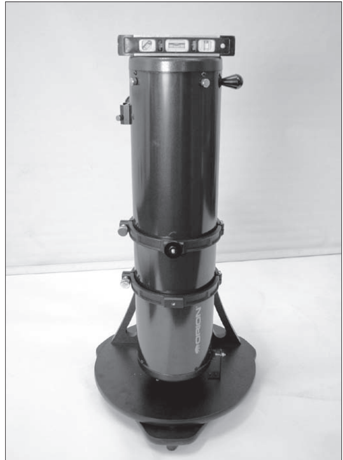
Figure 24. Once the base is leveled, point the optical tube up until the mirror cell (bottom end ring) contacts the vertical stop knob. Then place the carpenter's level across the top of the tube as shown and adjust the vertical stop knob until the tube is level. After each adjustment of the vertical stop knob, make sure to re-establish contact between the telescope end ring and the knob before checking the carpenter's level.
