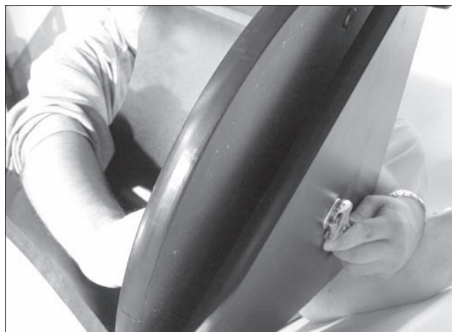
Figure 9. To reassemble the baseplates, tilt them only slightly, as shown. Do not place them on their side. Use one wrench to hold the azimuth axis bolt head steady while turning the hex lock nut with the other wrench.
