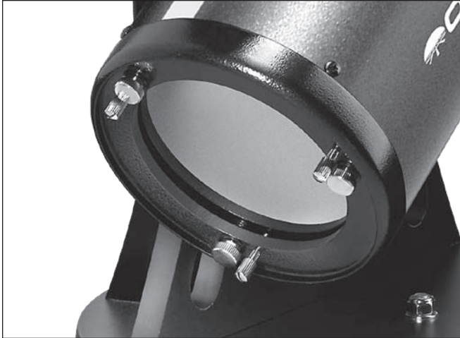
Figure 31. The collimation and mirror locking thumbscrews
