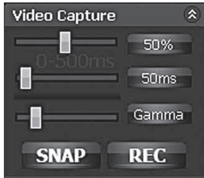
Figure 5: The video Capture interface showing Gain, Exposure and Gamma settings.
