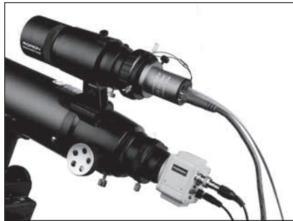
Figure 21. The SSAIO setup for guiding using the Orion Mini guider with helical focuser.
