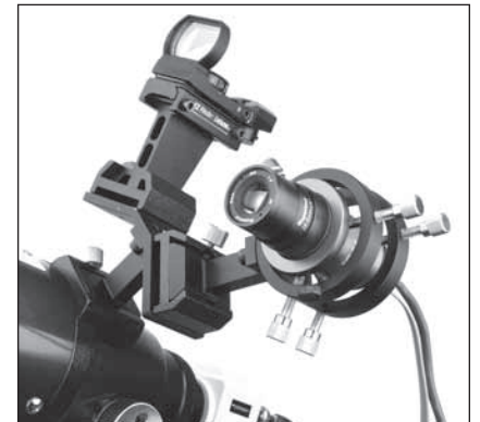
Figure 19: The SSAIO configured as a digital finder.
