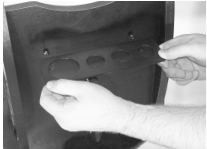
Figure 8. Using the two supplied screws, install the aluminum eyepiece rack in the predrilled holes near the top of the front baseplate.
