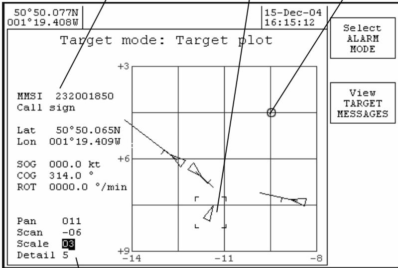
The display control section operates by selecting the desired field using the Navpad up and down keys, then using the Navpad left and right keys to change the parameter.
