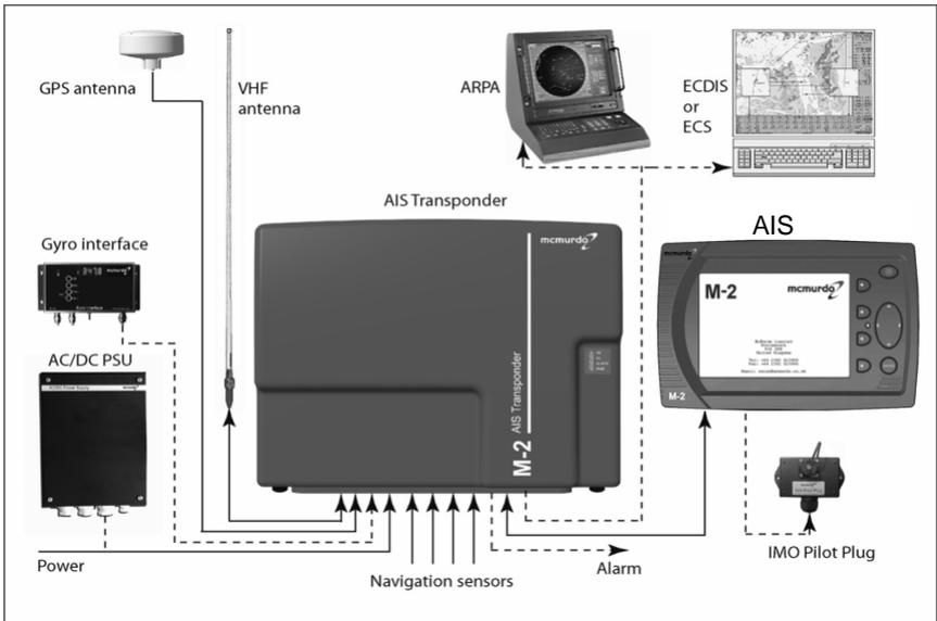
Comprehensive interfaces are provided for the connection of the vessel's primary navigation sensors, Integrated Bridge System (IBS) or Electronic Chart System (ECS).
