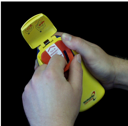
Pulling anti-tamper cover from PLB
