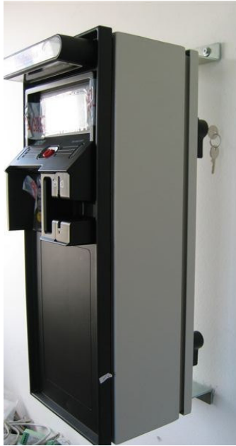
Figure 2-2. Secured OrPT Single Box – Wall Mounted
