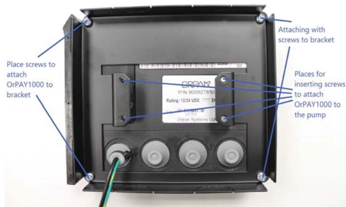
Figure 2-3 - OrPAY1000 Tightened to Bracket
