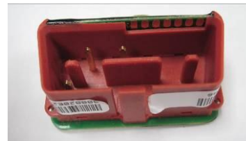
\mu DataPass (k-line) for K-line Protocol
