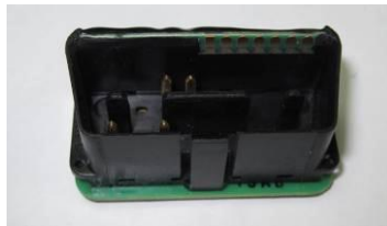
\mu DataPass (CAN) for CAN Bus Protocol
