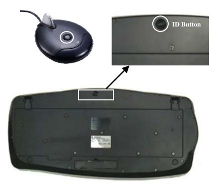
C. Press the ID button on the receiver first; then the receiver's ID LED will flash. Then press the ID button under the keyboard. The receiver's ID LED will accelerate flashing; it means the keyboard's setting up is completed.
