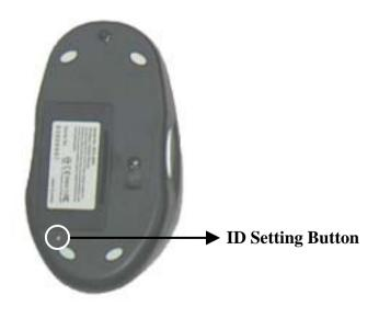
C. Press the ID button on the receiver first; then the receiver's ID LED will flash. Then press the ID button under the mouse. The receiver's ID LED will accelerate flashing; it means the mouse's setting up is completed.
