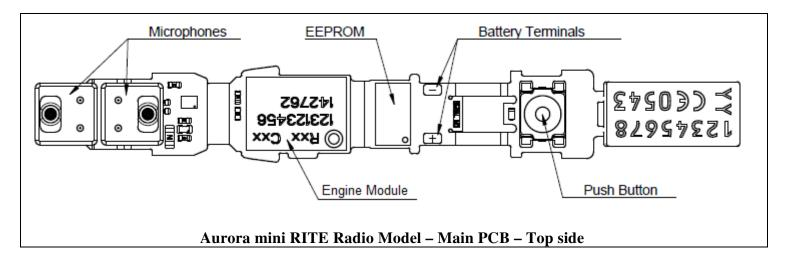
The most important part of the radio model is the Engine Module mounted on the main flex PCB, which connects it to both the EEPROM memory and all external connections: On the top side these are the microphones, the battery terminals and the push button.
