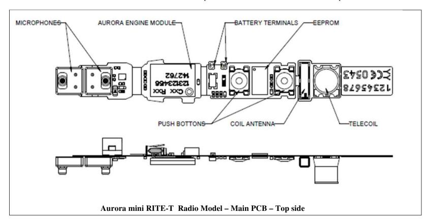
The most important part of the radio model is the Engine Module mounted on the main flex PCB, which connects it to both the EEPROM memory and all external connections: On the top side these are the microphones, the battery terminals and the push button.
