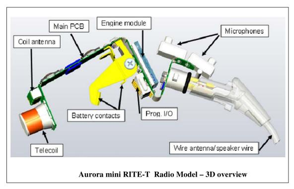
The radio model is implemented on the main PCB is shown to the left in 3D with connections to the antennas, the microphones, the speaker and the battery terminals.
