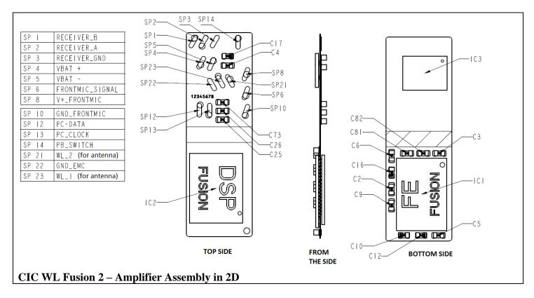
The module only requires a battery, an external microphone and speaker to be attached in order to run. All components are kept in place by the face plate as mechanical carrier for the radio model.
