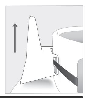
NOTE: For installations carried out as part of the TMAAS program, collar mounting with cable tie is mandatory.
