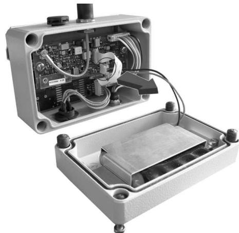
**Figure 4. Unplugging the PCB Connector**
