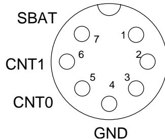
Figure 6. Pins on the I/O Connector (Top View)
