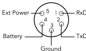
Figure 7. A724 POWER Connector (Top View)
