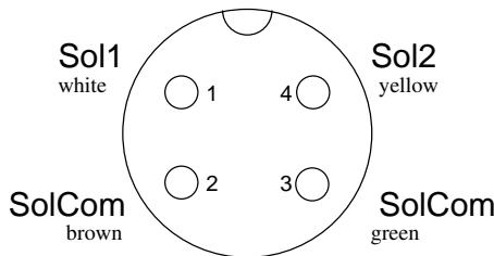
**Figure 11. The Valve Connector**
