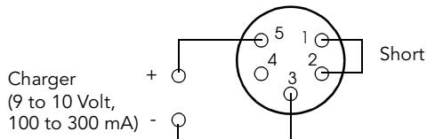
Figure 9. A724 Connection with External Power Supply
