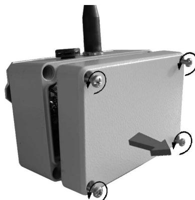
**Figure 3. Removing the addSWITCH Lid**
