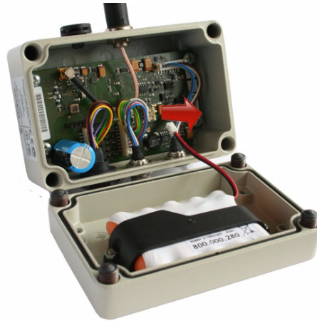
Figure 4. Unplugging the PCB Connector
