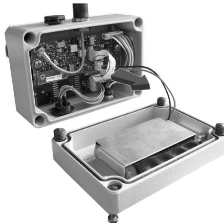
Figure 4. Unplugging the PCB Connector
