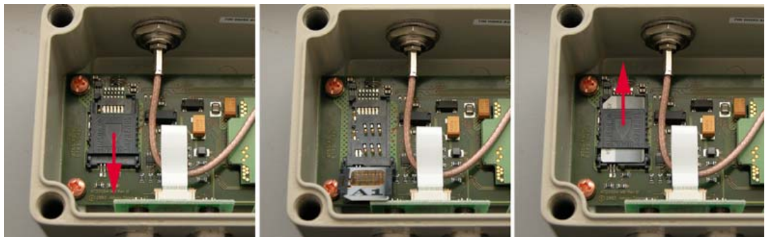
Fig. 4: Installing the SIM card in the A733GSM RTU
