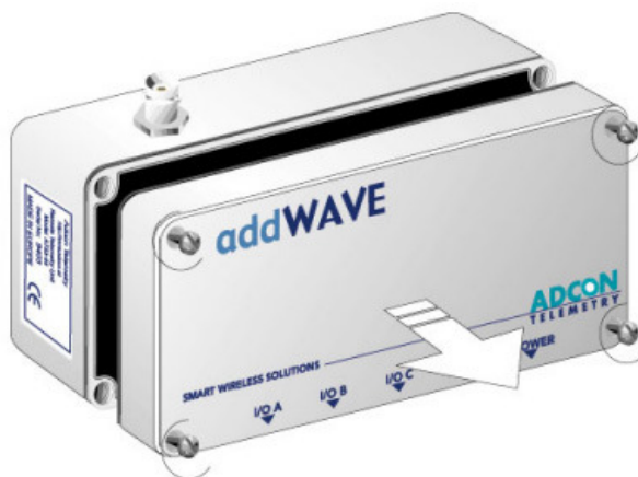
Figure 2. Lift the A753 lid
