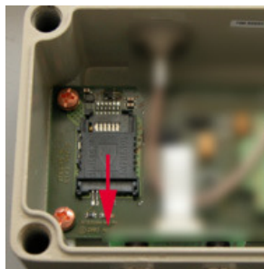
Figure 3. Open the SIM card holder
