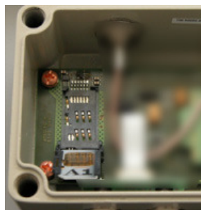
Figure 4. Insert the SIM card into the holder
