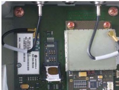
Figure 6. Insert the SIM Card into the Holder
