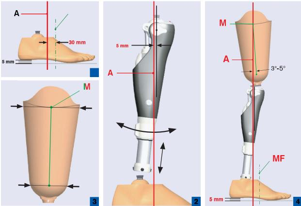
A correct bench alignment (e.g. using the 743L200 LASAR Assembly) ensures that the user can benefit from all the advantages of the C-Leg®. The residual limb position must be considered when positioning the socket connector. Plumb lines in the frontal and sagittal planes (drawn from the hip joint's center of rotation and marked during plaster cast taking and trial fitting of the test socket) will facilitate the correct positioning of the lamination anchor or socket adapter.
