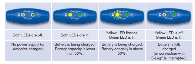
**4** After charging, remove the charging plug (C-Leg® performs self-test and activates 1st mode) and reattach the protective plug.
