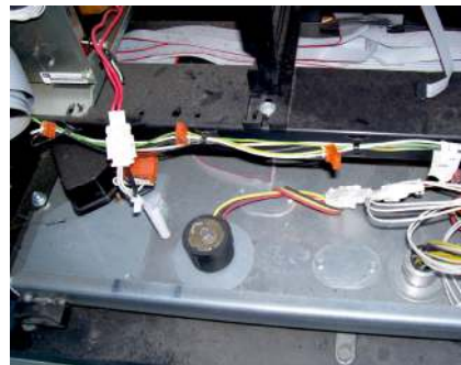
Illustration C.1: Sample Gilbarco dispenser AC buss.
