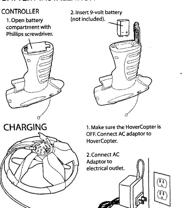
3. A full charge will take about 15 minutes. Fly the HoverCopter after each charge. Repeatedly charging without flying in between may damage the batteries or reduce their performance. Remove AC adaptor from electrical outlet after use.
