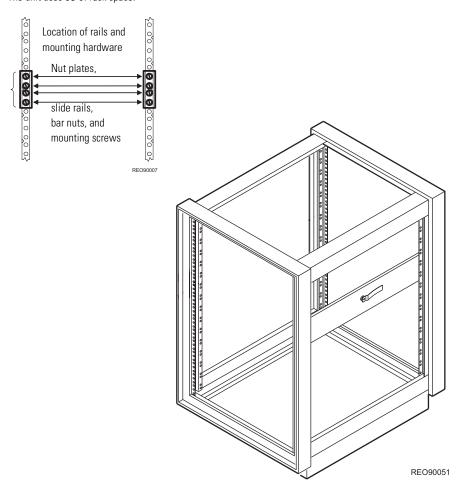
${f 3}$  Fasten each outer slide by using 10-32 screws (with washers, if needed) and one nut plate.
