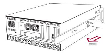
■ Continue to pull the outer slide towards the rear until the outer slide-lock engages the intermediate slide. To permit the intermediate slide to continue to move toward the rear, press the inner slide-lock button. Continue to move the outer and intermediate slides toward the rear until they are separated from the inner slide.
