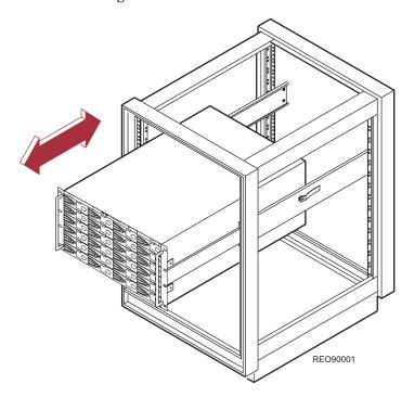
**9** Slide the REO Appliance into the rack, and attach the captive screw on each panel extension (left and right sides) to the rack and nut plate.
