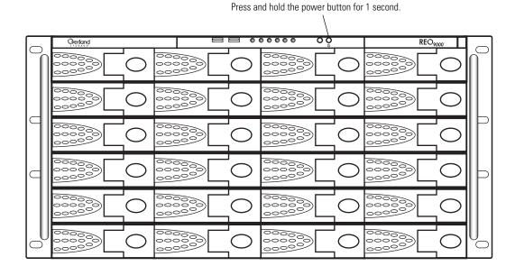
After you turn the power on, the REO Appliance performs a self-test process and loads the necessary information from the REO SoftKey. Following successful completion of the self-test, which takes several minutes, you should hear 3 beep tones.
