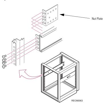
Note: When fastening the adjustable bracket, allow room for the slide to pass by the inside of the rack.
