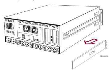
**2** Locate the screw holes in the front and rear rails of the rack where the REO Appliance slides will be installed.
