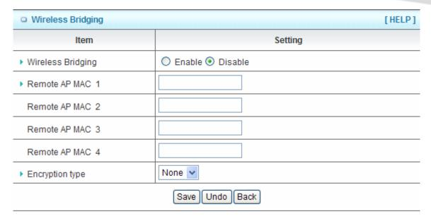
Wireless Bridging: You could enable this function by selecting "Enable".
