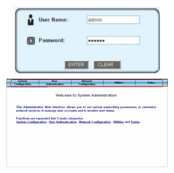
**Manager:** The manager can only access the configuration pages under *User Authentication* to manage the user accounts, but has no permission to change the settings of the profiles for Firewall, Specific Route and Schedule.
