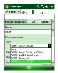
6. Tap the Port dropdown list and select the COM-port previously assigned to the X-MET8000 Series
