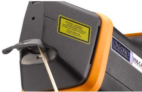
Cleaning the measurement window with a cotton bud
