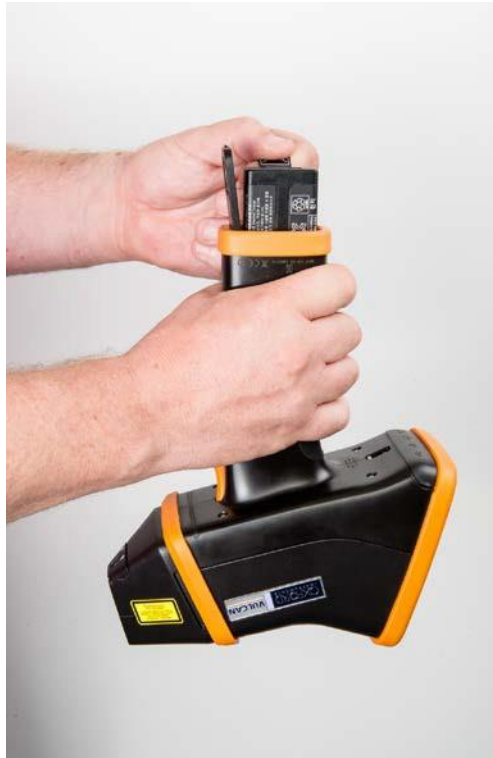
Pulling the battery out of the battery compartment
