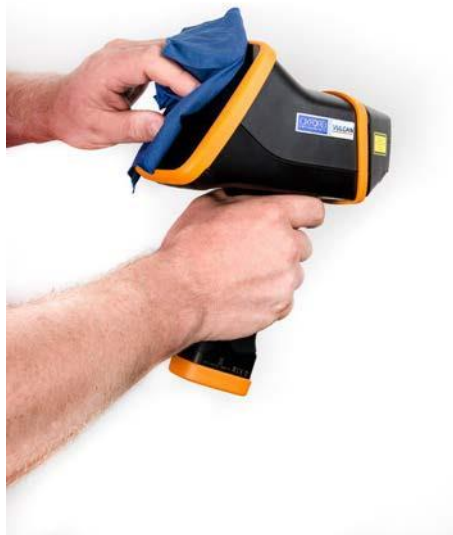
Wiping the instrument housing clean with a piece of cloth and mild detergent
