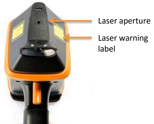
The analyzer nose showing the groove on the sides of the and indicating the center of the laser spot.
