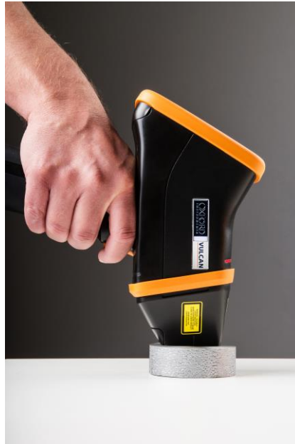
Analyzer nose in contact with the sample
