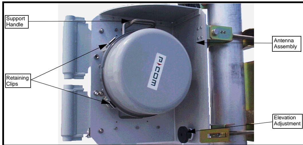
Figure 6-6 - Attaching ODU to Antenna Mount Assembly
